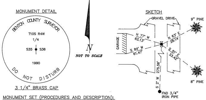
SET: 2" INSIDE DIAMETER BY 36" LONG IRON PIPE WITH A 3 1/4" BENTON COUNTY BRASS CAP, STAMPED AS SHOWN, IN THE SAME POSITION AS THE STRAIGHT BASE OF THE RECOVERED 1" IRON PIPE. BURIED THE 1" PIPE HORIZONTALLY ALONG THE EAST SIDE.
