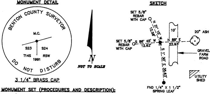
SET: 2" INSIDE DIAMETER X 36" LONG IRON PIPE WITH A 3 1/4" BENTON COUNTY BRASS CAP, STAMPED AS SHOWN, CENTERED OVER THE RECOVERED 7/8" IRON ROD.
